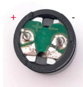
We can make recognizable notes by getting the passive buzzer to click hundreds of times a second at a particular frequency, so first we need to know the frequency of the different tones we want. The following table shows the notes and their corresponding frequencies. Period is the duration of the cycle, in microseconds, at which the frequency is created. For example, to get a C note (261 Hz), we need the piezo to cycle at a period of 3,830 microseconds.
