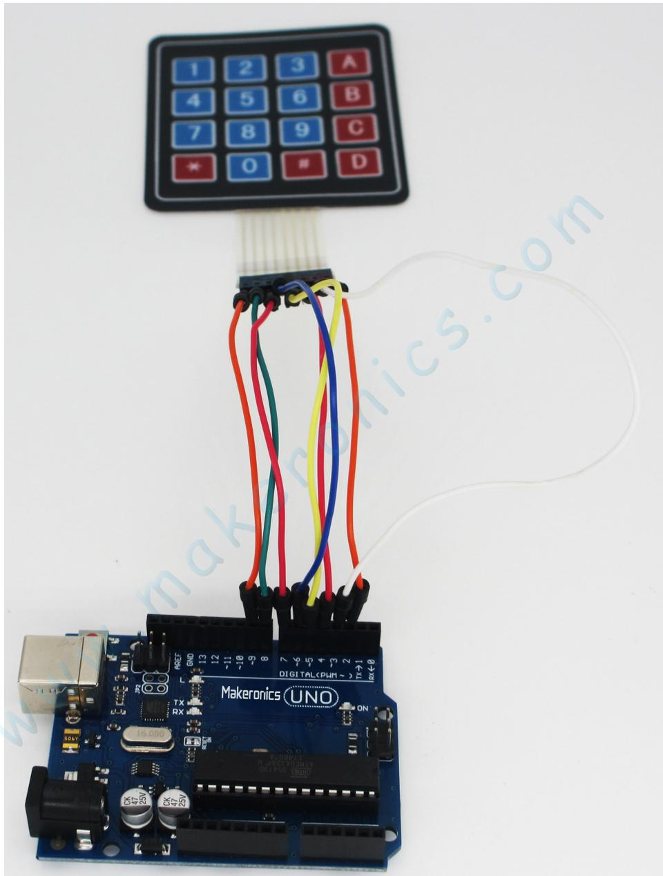
With this code, once we press a key on the keypad, it should show up on the serial monitor of the Arduino software once the code is compiled and uploaded to the UNO R3 board. Click the Serial Monitor button to turn on the serial monitor. The basics about the serial monitor are introduced in details in Lesson 2.
